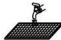
4—wash the pre-filter under running water
